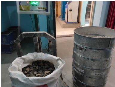
Fig. 1. Crushing test conducted on aggregates
