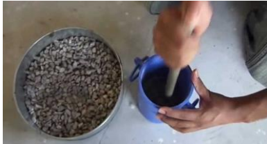
Fig. 1. Crushing test conducted on aggregates
