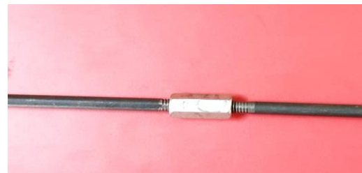
Fig. 5. Splice (Coupler) lapping
