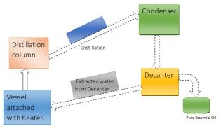
Fig. 4. Hydro distillation process
