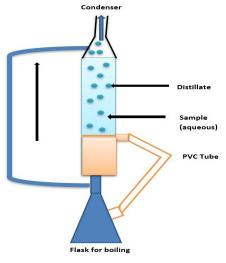
Fig. 3. Soxhlet extraction process
