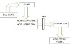
Fig. 1. CO<sub>2</sub> extraction process
