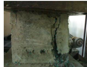
Fig. 5. Paper pulp based concrete cube failure
