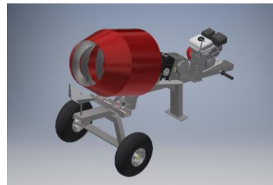
Fig. 2. Molen machine design capacity 0.065 m 3
