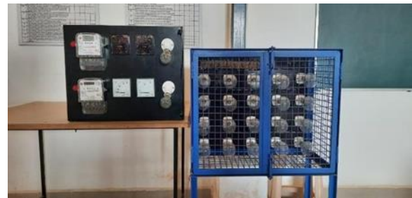
Fig. 2. Calibration of single-phase energy meter actual model
