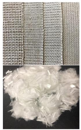
Fig. 2. Textile reinforcement
