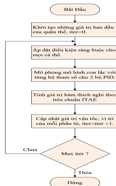
Fig. 6. Algorithm flowchart of PSO-PID control system
