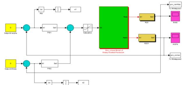
Fig. 3. Control diagram to keep the balance of the forward pendulum for both angles  $\alpha$  and  $\theta$
