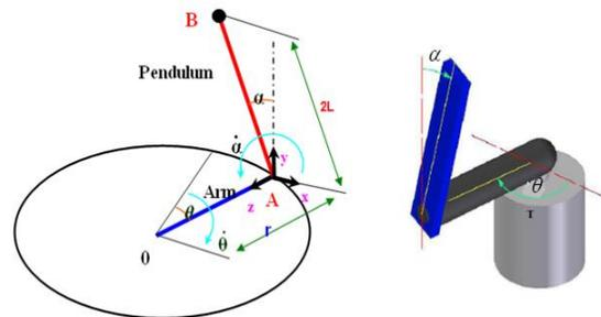
Fig. 1. Simple model of an inverted pendulum
