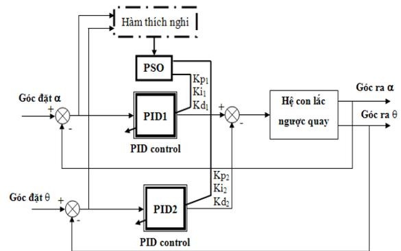
Fig. 5. PSO-PID control system
