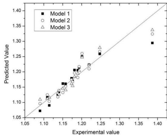
Fig. 10. Prediction of TCR for TiO<sub>2</sub>-Ag/distilled water
