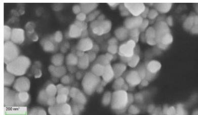
Fig. 2. FESEM image of  $\text{TiO}_2$  - Ag nanocomposite
