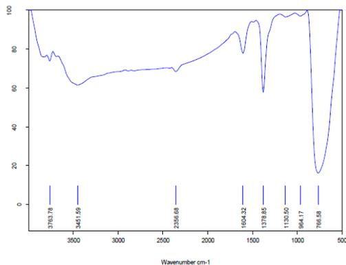
Fig. 5. FT-IR spectrum of  $\text{TiO}_2$ -Ag nanocomposite particle
