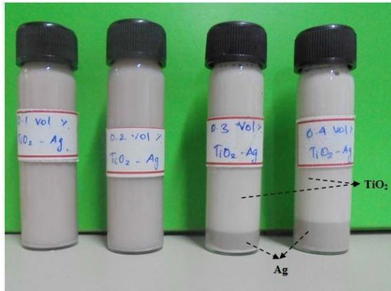
Fig. 8. Disassociation in TiO<sub>2</sub>-Ag/distilled water
