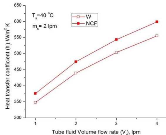
Fig. 13. Heat transfer coefficient for different tube fluid volume flow rates
