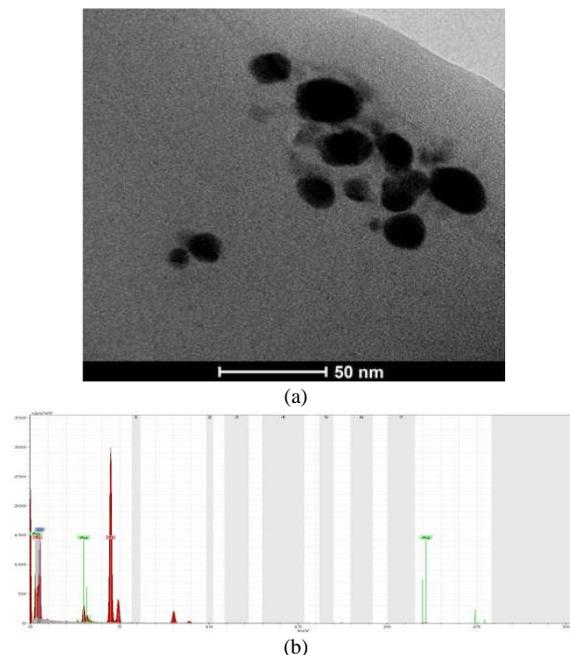
Fig. 3. (a) HRTEM image of  $\text{TiO}_2$ -Ag nanocomposite particle and (b) EDAX spectra of  $\text{TiO}_2$ -Ag nanocomposite particle
