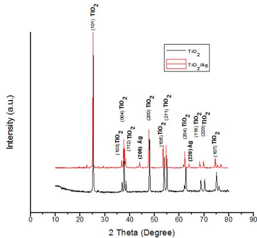
Fig. 4. XRD image of  $\text{TiO}_2$ -Ag nanocomposite particle
