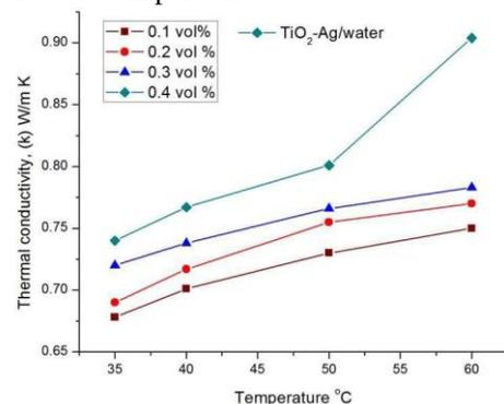
Fig. 7. Thermal conductivity for  $\text{TiO}_2$ -Ag/distilled water
