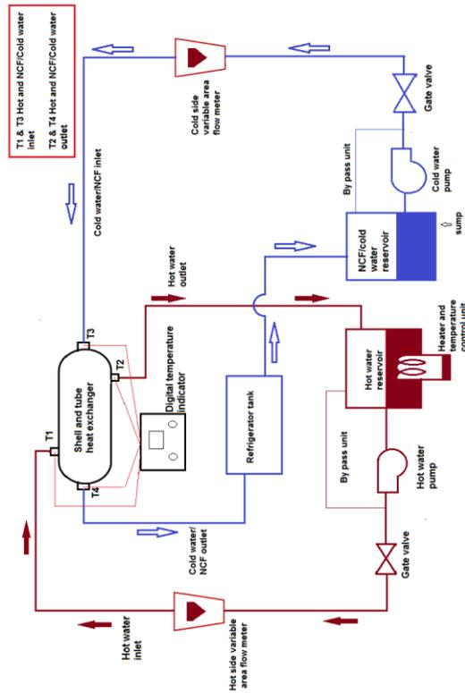
Fig. 11. Schematic view of shell and tube heat exchanger experimental set up
