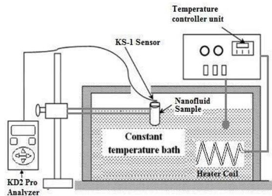
Fig. 6. Thermal conductivity measuring unit
