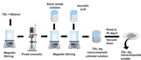
Fig. 1. Synthesis of  $\text{TiO}_2$ -Ag nanocomposite particle
