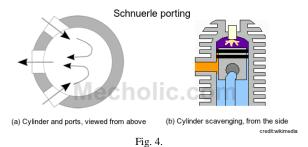
Similar to the cross flow scavenging but the inlet exhaust port is replaced the same side of the engine cylinder the gases are encouraged to move loops this type of scavenging use carefully designed transfer port to loop fresh air rise towards the cylinder head on one side and pushes the burnt gas down to the exhaust
