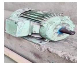
Fig. 3. 3 phase I.M, 1 HP Squirrel cage
