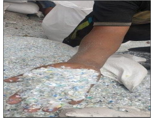
Fig. 2. Shredded HDPE waste plastic passing sieve 2.36mm and retained 600 micron sieve
