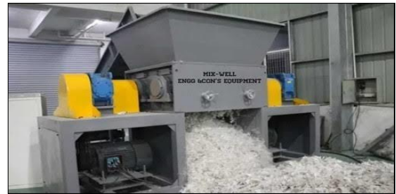
Fig. 3. Plastic shredding machine
