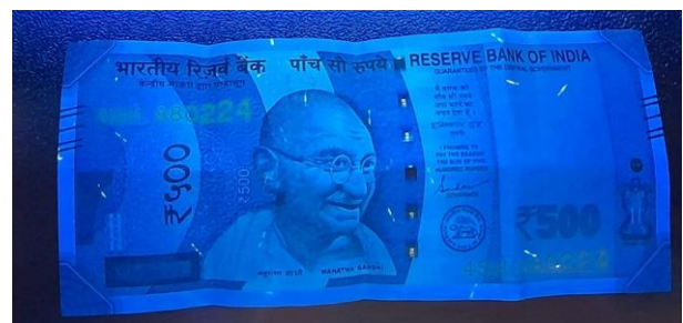
Fig. 1. It is the front side of 500 Rupee note. Under Ultraviolet Light source we can easily see the different security threads present inside the 500 note which are scattered non-uniformly along with all other features as mentioned in table 1
