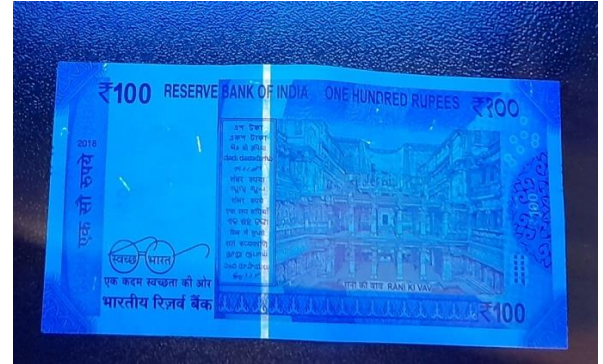
Fig. 3. These are some more photographs of 20 and 100 rupee note, both front and back side to observe security features of Indian Currency Notes under Ultraviolet light source as mentioned in table 1
