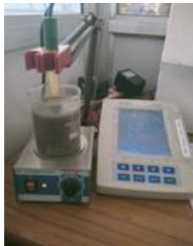
Fig. 2. 150ml of Calcium hydroxide + Rice husk
