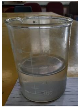
Fig. 5. 250ml of distilled water + 1gm CAO + 1gm Rice husk ash
