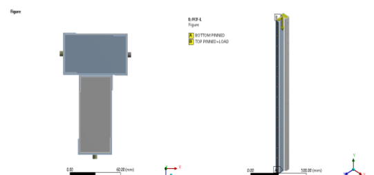
Fig. 11. Model and boundary condition diagram of FCF-T
