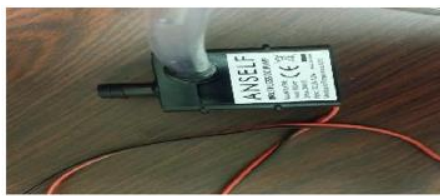
Fig. 7. DC water pump (12V/4.2 W)
