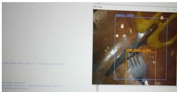
Fig. 5. The objects are detected as scissors and metal object with confidence value of 0.834 (83.4%) and 0.7940 (79.40%) respectively, Here the real time code is executed
