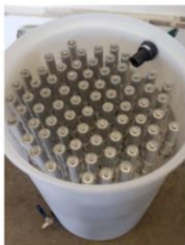
Fig. 3. Thermal energy storage tank fully assembled with all PCM inserted
