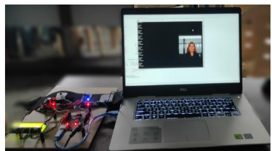
Fig. 10(b). The results which are displayed from the facial landmark is happy and the outcome displayed by the stress meter for this person is ‘NOT STRESSED’
