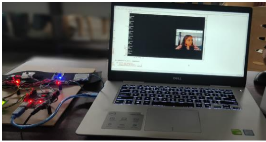
Fig. 10(c). The results which are displayed from the facial landmark is sad and the outcome displayed by the stress meter for this person is 'STRESSED'
