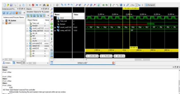
Fig. 6. Simulation result when watchdog timer reset and restart received from controller
