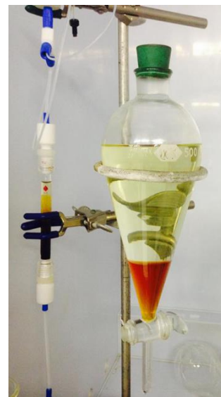
Fig. 5. Two Phase Separation and Resin Column
