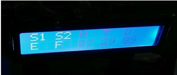
Fig. 8. LCD display showing slot1 empty and slot2 filled
