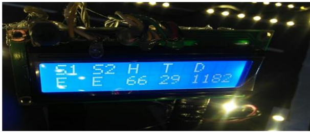
Fig. 7. LCD display showing both the slots are empty
